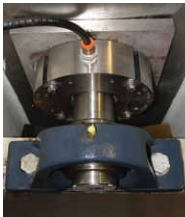
The stainless steel food grade Inpro/Seal® Air Mizer® is a permanent shaft sealing solution that meets all FDA requirements.
